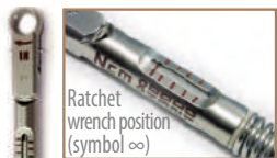
Torque wrench position (10 to 45 N.cm)
